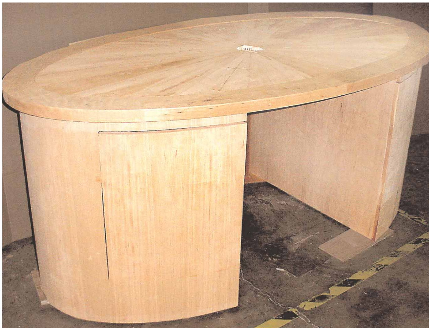
The roughed pieces are stacked for inspection before the shelf-and-drawer combinations are attached. The design of this top was scrapped in favor of a simpler, four-part inlay that displayed the grain to best advantage.
