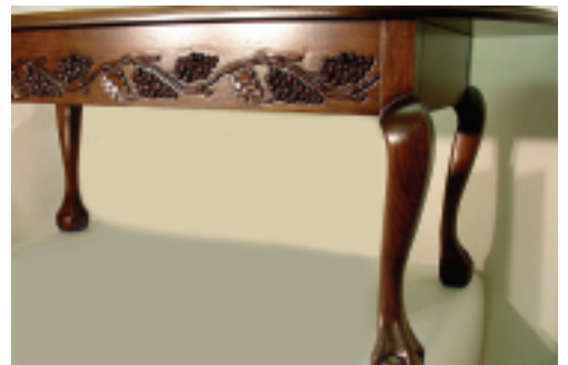
Harbaugh shows off the coffee table apron which was carved on the school's Thermwood CNC router using ArtCAM V6 software from Delcam.
